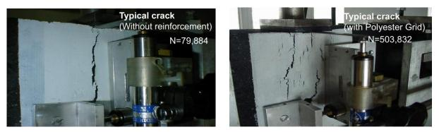
FIGURE 3c. Comparison of Beams with and without PET grid: Typical Cracking Patterns and the Number of Cycles Conducted Before the Cracks Reached the Surface (Bending and Shear mode) [1]
