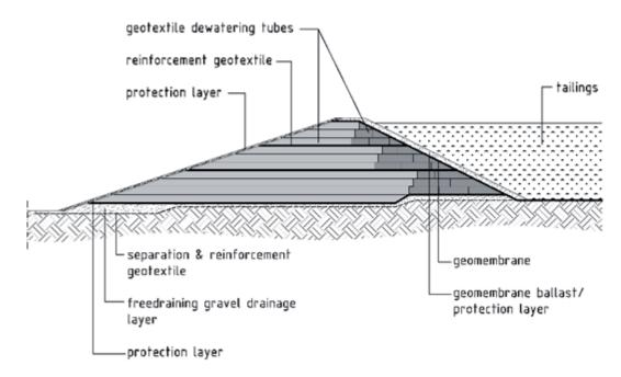
Figure 4. Construction Concept: Dewatering tube tailings dams
