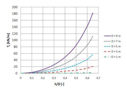
Figure 3. Tensile strength as a function on filling ratio, Wilke & Hangen (2011)
