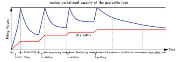
Figure 2. Schematic diagram of the dewatering sequence with geotextile tubes, Wilke & Breytenbach (2016)
