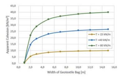
Figure 6. Apparent cohesion calculated using Eq. 1 depending on width of geotextile bags, H =  $2,0 \text{ m}. \phi^2 = 20^\circ$
