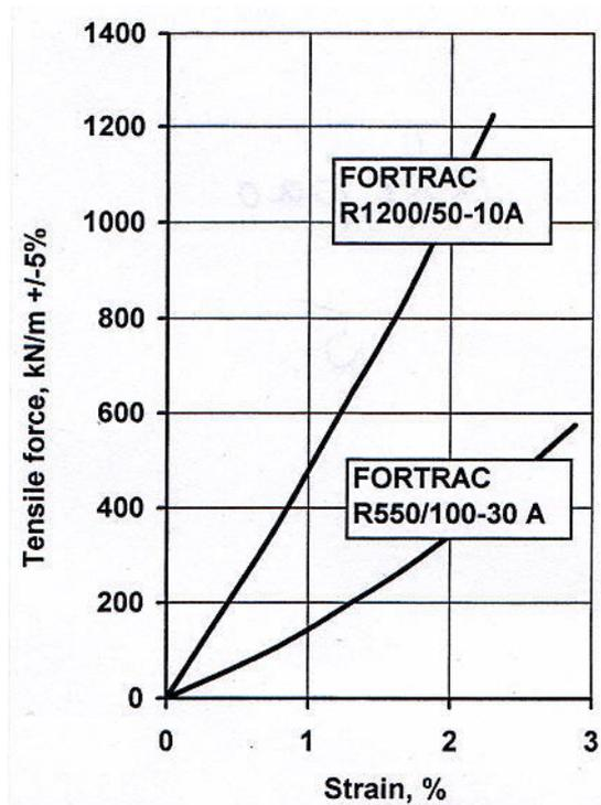
Figure 5. Stress-strain curves (short-term) of the aramid geogrids for the Böschtobel landfill
