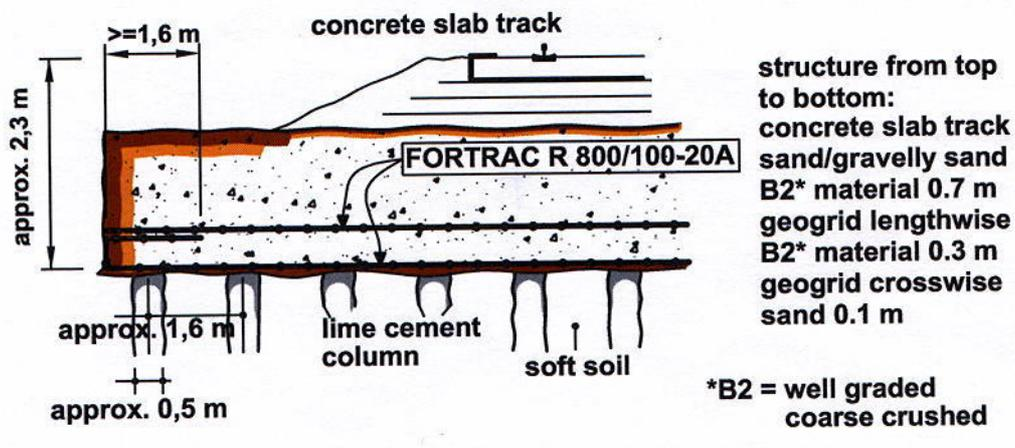
Figure 7. German Railways ICE high-speed line Hanover-Berlin, aramid geogrids on cemented stone columns at Rathenow ('Körgraben')
