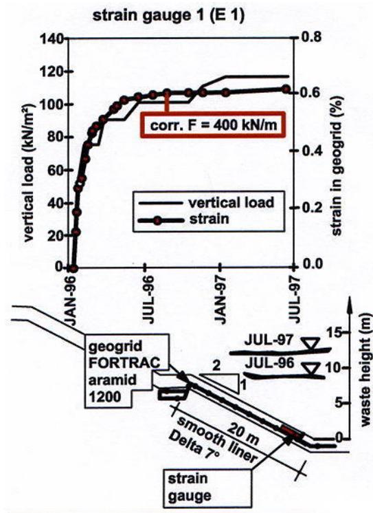
Figure 6. Typical measurement results from a cross-section at the Böschistobel landfill
