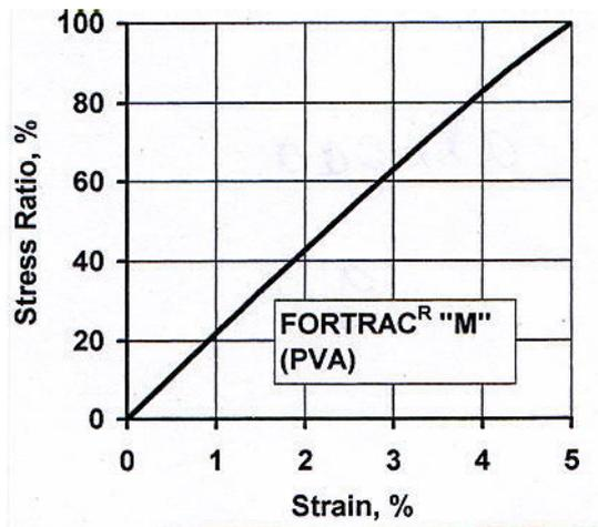
Figure 9. Typical stress-strain short-term curve for the PVA-geogrids described
