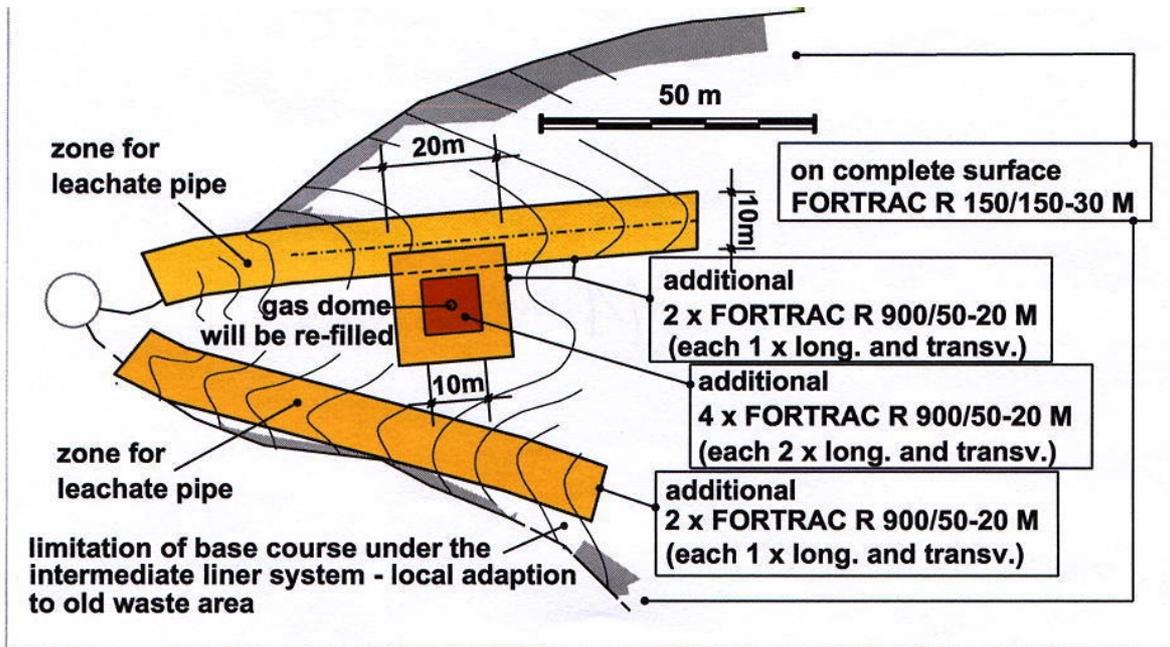
Figure 11. Einöd landfill, reinforcement of the base for the intermediate seal with PVA geogrids
