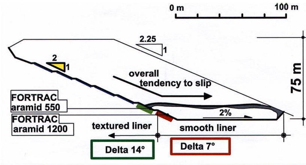
Figure 4. Illustration of the problem “anti-sliding reinforcement” of the Böschistobel landfill in Austria
