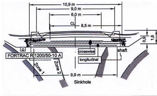
Figure 2. Cross section of the Federal Road B 180: geogrid in transverse direction with large turn-back to provide additional torsional resistance
