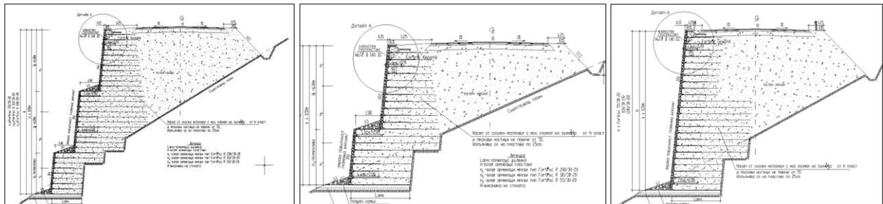
Figure 3. Concepts for typical cross-sections: front (facing) inclination always 10v:1h, but different number of berms.
