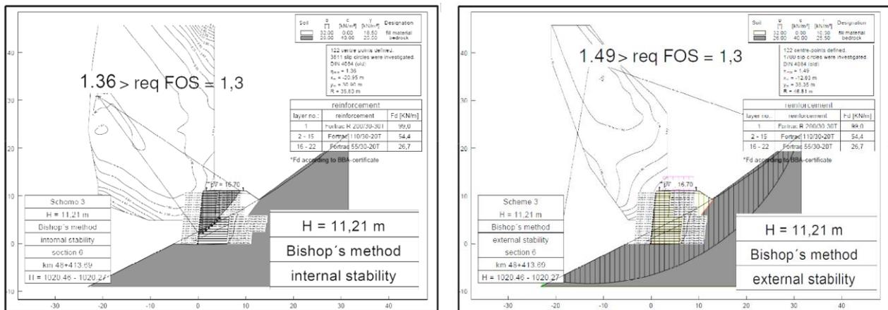
Figure 6. Typical examples of stability analyses according to Bishop (“internal” to the left, “external” to the right).
