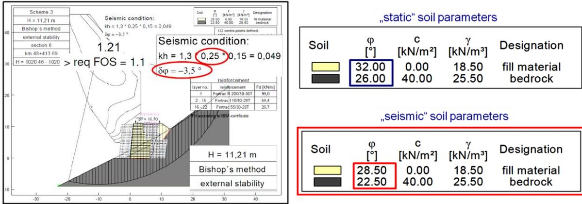
Figure 8. Seismic external stability analysis for the cross-section in Figure 6 (left); and assumed soil parameters right.
